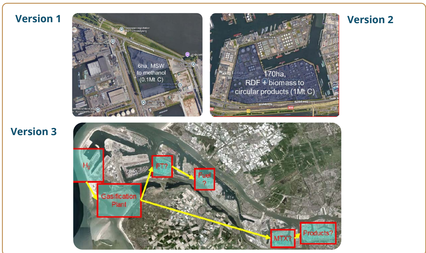
Figure 3: Impression of a Version 1 plot, a Version 2 site, and Version 3 cluster-wide ecosystem of distributed sites connected by syngas infrastructure, projected on the HIC.
